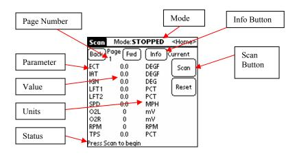
To start scanning, click the "Scan" button on the screen, or press the Page-Up button. The mode at the top of the screen should change from "Stopped" to "Scanning", and you should see some values display on the screen. If you see "T.O." instead, that means there's been a timeout error (no response from vehicle). Double-check the cables are all in place & the vehicle key is "on".
